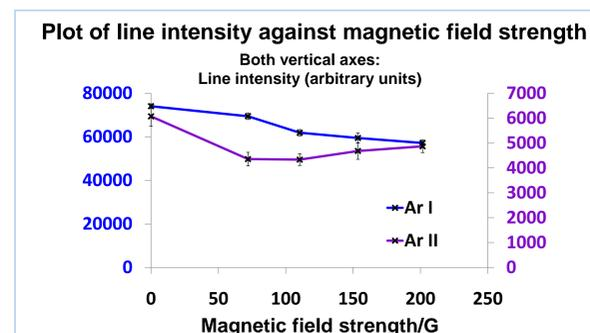
Figure 7: Plot showing the effect of introducing a magnetic field on the brightness. Lines used: Ar I 696.5 nm; Ar II 434.8nm
