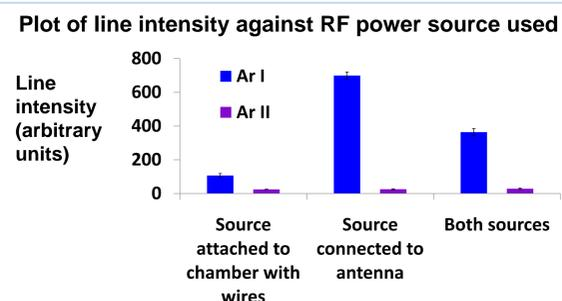
Figure 4: Plot showing the effect of changing the RF source powering the plasma on the brightness. Lines used: Ar I 696.5nm; Ar II 611.5nm
