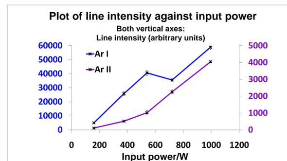
Figure 6: Plot showing the effect of changing the input power on the brightness. Lines used: Ar I 696.5nm; Ar II 434.8nm
