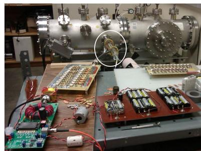
Figure 2: Image of vacuum chamber (silver, in the background); plasma tube (circled); and controlling circuitry (foreground)
