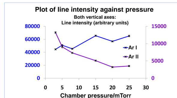
Figure 5: Plot showing the effect of changing the pressure in the plasma chamber on the brightness. Lines used: Ar I 696.5nm; Ar II 434.8nm
